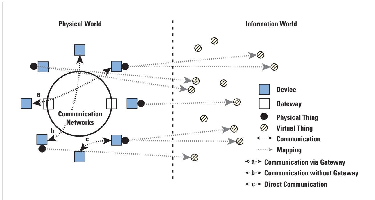
Figure 3 introduces one additional IoT-related device: the *gateway*. At minimum, a gateway functions as a protocol translator. Gateways address one of the greatest challenges in designing an IoT, which is connectivity, both among devices and between devices and the Internet or enterprise network. Smart devices support a wide variety of wireless and wired transmission technologies and networking protocols. Further, these devices typically have limited processing capability.
