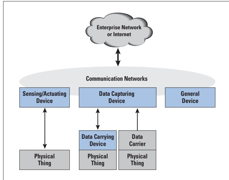
The model makes a distinction between data-carrying devices and data carriers. A data-carrying device is a device in the Recommendation Y.2060 sense. A device at minimum is capable of communication and may include other electronic capabilities. An example of a data-carrying device is an RFID tag. By contrast, a data carrier is an element attached to a physical thing for the purpose of identification or providing some other sort of information.
