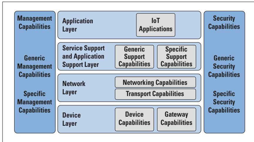
The *Network Layer* performs two basic functions. Networking capabilities refer to the interconnection of devices and gateways. Transport capabilities refer to the transport of IoT service- and application-specific information as well as IoT-related control and management information. Roughly, these capabilities correspond to those of the OSI network and transport layers.
